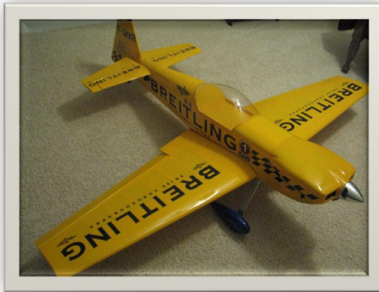
CAP 231: This beautiful 30CC size CAP belongs to our fellow club member, Ben Davis. Comes in ARF form manufactured by SIG. It was assembled by Gary Elliott. It was fitted with an Evolution 26cc gas engine.
