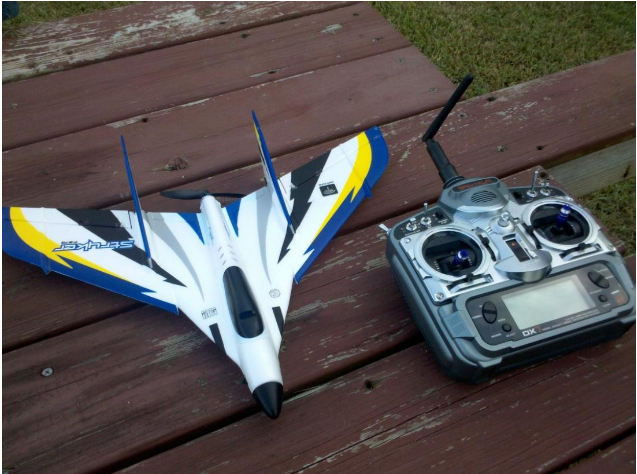
New Parkzone UMX Stryker F27Q flown with a DX 7. You do need a programmable radio to fly it.
