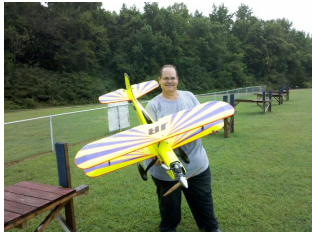
My (Dr. Joey) new Hog Bipe. Has a 20cc gas 4 stroke Saito FG20 with 9 servos. Electronic Ignition. Maiden flight by J.T. Builder: Gary Elliott Manufacturer: SIG Weight: 10 \frac{3}{4} pounds = 2 bricks. The sound of the 4 stroke is nice. The fuel efficiency is great with 45 minute flights in 12 ounces of gas. Ignition battery and receiver battery are 1600mah 6 volts each. Flies really nice.
