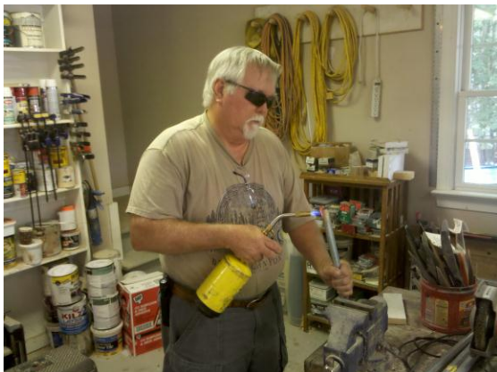
J.T. is getting ready some metal tubing to bury in the field between airplane stands. Then you can insert a fork holder to hold the rear of your airplane when you want to start the engine on the ground. This was done on the last work day at the field a couple of weeks ago.
