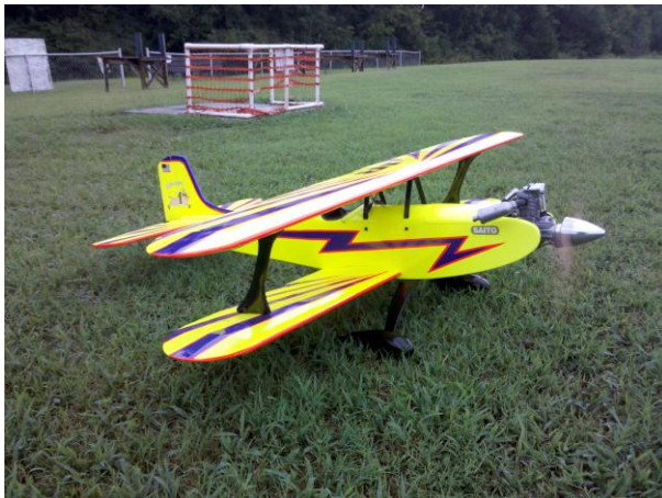
My (Dr. Joey) new Hog Bipe. Has a 20cc gas 4 stroke Saito FG20 with 9 servos. Electronic Ignition. Maiden flight by J.T. Builder: Gary Elliott Manufacturer: SIG Weight: 10 \frac{3}{4} pounds = 2 bricks. The sound of the 4 stroke is nice. The fuel efficiency is great with 45 minute flights in 12 ounces of gas. Ignition battery and receiver battery are 1600mah 6 volts each. Flies really nice.
